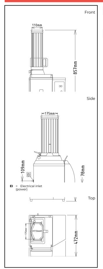
Electric Supply voltage: 601589 (DCPXF215) 220-240 V/1N ph/50 Hz 0.37 kW **Total Watts:** Key Information: External dimensions, Width: 472 mm External dimensions, 418 mm Depth: External dimensions, 857 mm Height: Net weight (kg): ISO 9001; ISO 14001
